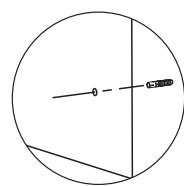
2. Mount the letterbox onto the brickwork with the washers and screws/bolts provided.
